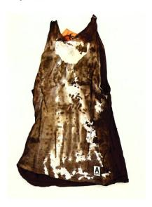
One hole lacked characteristics to determine the type of fabric damage or the possible source. One hole was consistent with puncture-like damage. It was determined that this hole could have been made by a taser probe. See below for summarized chart:
